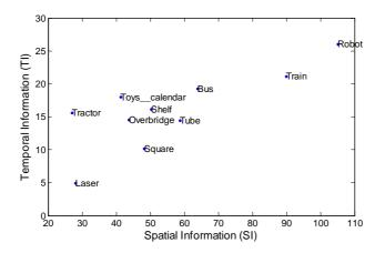
Figure 2. The distribution of content complexity of source video contents. The SI and TI are calculated according to ITU-T P.910.
